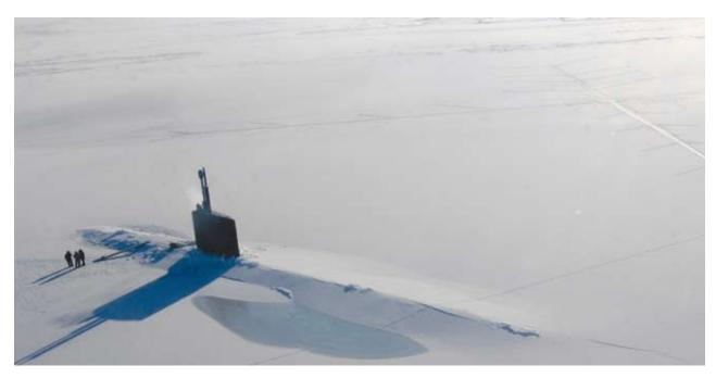
The Los Angeles-class submarine USS Annapolis (SSN 760) broke through three feet of ice during Ice Exercise (ICEX) 2009 in the Arctic Ocean. ICEX 2009 was intended to test and evaluate naval submarine operability in the changing Arctic environment. (MASS COMMUNICATION SPECIALIST 1ST CLASS TIFFINI M. JONES/U.S. Navy)
