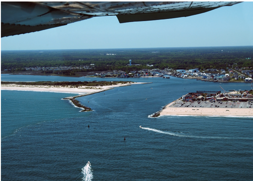
Figure 29. Oblique aerial photograph of Ocean City Inlet in the Delmarva North region. Assateague Island (on the left) has migrated more than 500 meters since the inlet was stabilized in the 1930s. Ocean City, MD, is on the north side of the inlet.
