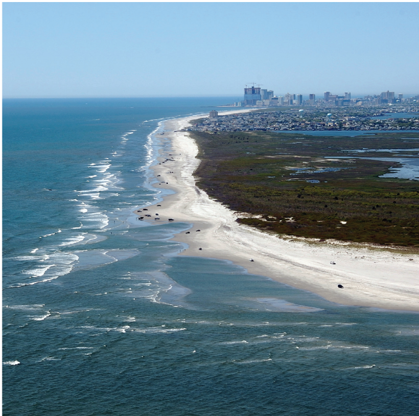
Figure 27. Oblique aerial photograph at Brigantine Inlet, looking south toward Atlantic City, NJ. This is the location of the maximum short-term erosion rate (-19.3 meters per year) in the New Jersey South region.
